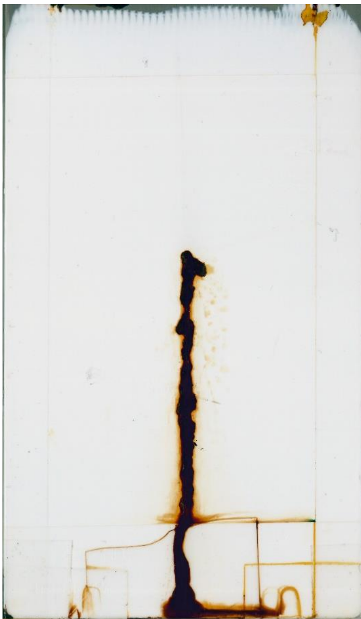
1440h NSST, Gardobond OC panel, approx. 110µm DFT
